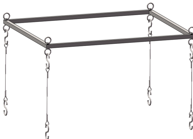
Figure 13: Lifting Tool for MYTEX U1L Modules
